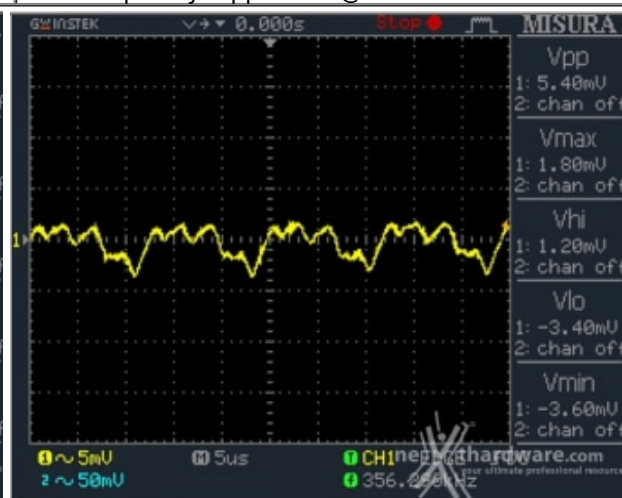
PWM Frequency Ripple 12V @ 0%
