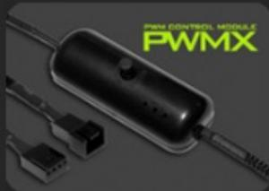
The brand new **PWMX-fancontroller**, enabling every conventional 3-pin fan to be controlled via PWM signals from modern mainboards. The PWMX translates the PWM signal so the fan will adjust rotation speed according to computer load, e.g. for enabling PWM support for conventional CPU or case fans. Furthermore, the PWMX controller allows adjustment of fan rotation maximum speed for optimal performance.
