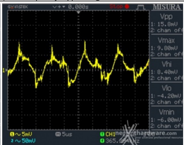
PWM Frequency Ripple 5V @ 0%
