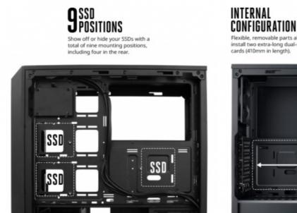
Flexible, removable parts allows you to install two extra-long dual-slot graphics
