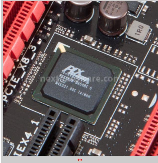
Il Bridge PLX collegato al Platform Controller HUB Z77.
