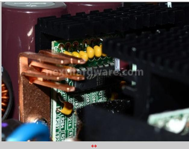
Particolare del Controller PWM [CM6800AG](http://pdf1.alldatasheet.com/datasheet-pdf/view/228693/CHAMP/CM6800AG.PDF) (<http://pdf1.alldatasheet.com/datasheet-pdf/view/228693/CHAMP/CM6800AG.PDF>).
