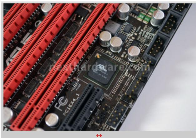
Bridge PLX collegato al Platform Controller HUB Z68.
