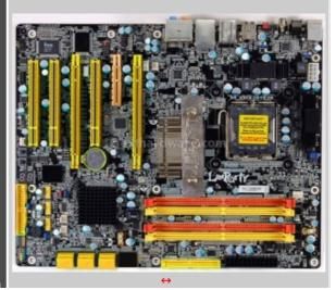
up to 3 Gbps and it supports RAID 0/ 1/ 0+1/ 5 as well. **High Definition 8 channels Audio**: the Realtek ALC885 codec is fully verified by Windows Vista Premium version.
