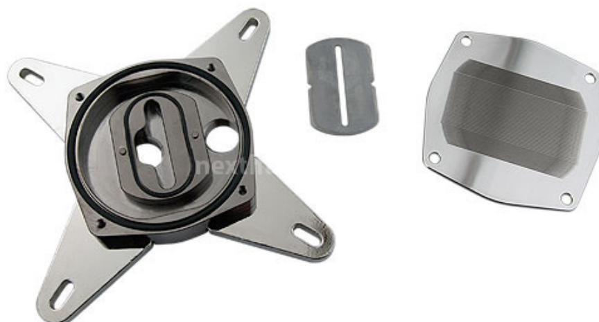
Koolance CPU-370 Microfin Cold Plate (0.25mm fins, 0.30mm channels)
