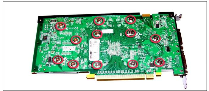
**7.** Turn the card on its back and remove the 12 screws highlighted above.
