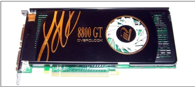
**6.** Before handing the card you should take precautions to avoid static damage. Remove the 8800 card from the box ready for installation.
