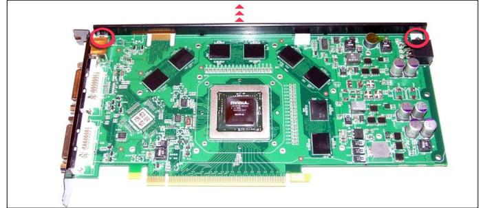
**9.** Unscrew the two screws highlighted above and remove the black aluminium bar. Clean the thermal paste from the GPU core ready for installation. When using thermal pads remember to remove the tape from both sides.
